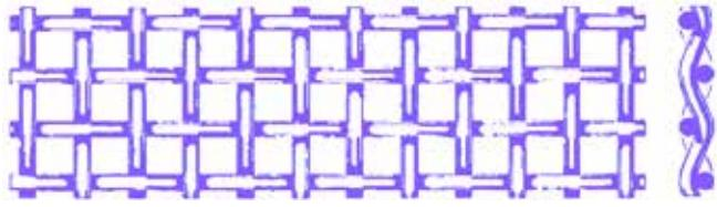
**PLAIN WEAVE** is woven from wires of the same diameter for both warp and weft, arranged in a symmetrical "over one and under one" pattern to provide square openings of precise dimensions. Plain mesh has great dimensional stability.
