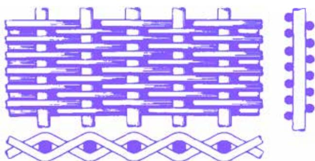
**HOLLANDER (DUTCH) WEAVE** is made with relatively thin weft wires packed closely together, and thicker more widely spaced warp wires. It resembles a 'basket' weave and does not have square apertures. Dimensionally very stable and having high bursting strength, it is suitable for pressure filtration where a large open area is not required.
