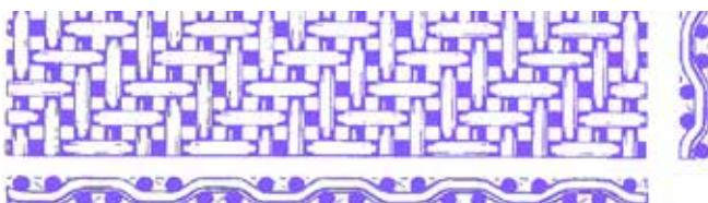
**TWILL WEAVE** is woven so that the individual wires in one direction pass over two and under the next two cross wires. It is less rigid than plain weave and is often used in very fine meshes.
